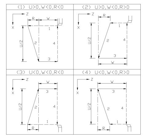
When symbols of R and W are inconsistent with each other, if |R| > |W|, the system will alarm as "1268-G90, G92 and G94 program error", meaning R value has exceeded the permitted range.
