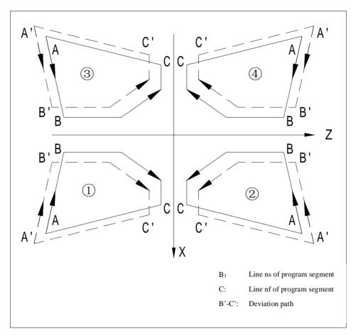
1)  $\triangle$ i can be set through the parameter (116-G73 allowance on axis X), and the set value can be modified through the program instruction. When  $\triangle$ i smaller than  $\triangle$ u, the system will alarm.
