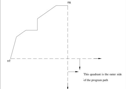
8)The deviation direction of rough-machining is determined by the program path: (The program path of machining is  $A \rightarrow B \rightarrow C$ ).
