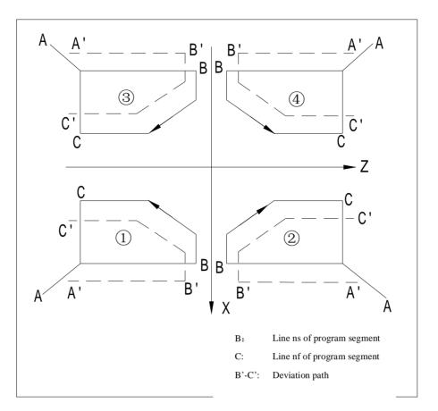
1)  $\Delta d$  can be set through the parameter (100-G72 feed of rough-machining cycle), and the set value can be modified through the program instruction. When  $\Delta d$  is 0 or higher than the total cutting output, the system will alarm.
