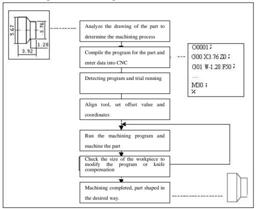
Figure 1 Process flow of CNC machining
