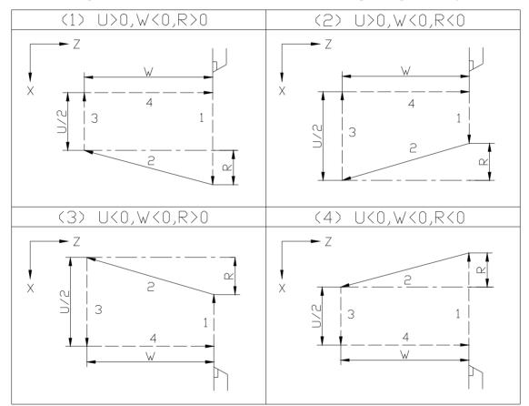
When symbols of R and U are inconsistent with each other, if |R| > |U/2|, the system will alarm as "1268-G90, G92 and G94 program error", meaning R value has exceeded the permitted range.
