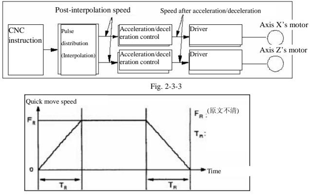
Fig. 2-3-4 Curve of Quick Move Speed
