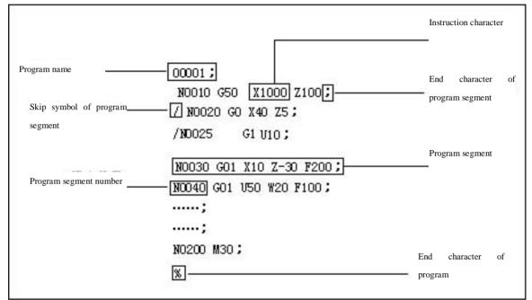
Fig. 1-3-2 Regular Structure of a Program
