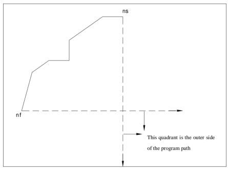
7) The deviation direction of rough-machining is determined by the program path: (The program path of machining is  $A \rightarrow B \rightarrow C$ ).
