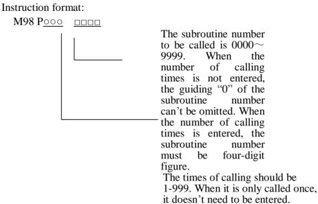
Definition: When other instructions of the program segment are executed, the system won't execute the next program segment, but the program segment designated by P. A subroutine can only be executed for 999 times at maximum. In MDI state, the subroutine can't be called.
