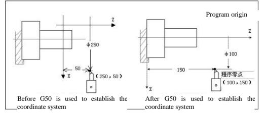
As shown in the above figure, after the instruction segment "G50 X100 Z150" is executed, the workpiece's coordinate system will be established and the point X100,Z150) considered the program origin.
