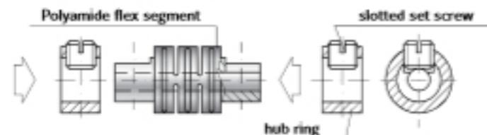
The screw threads through the clamping ring, through a slot in the flexible segment, and down onto the shaft, securing the entire assembly. Including a flat on the shaft can improve torque transmission.
