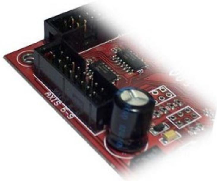
This connector controls up to 5 motor drivers. It can also provide an ENABLE signal to drivers that can take advantage of these feature.
