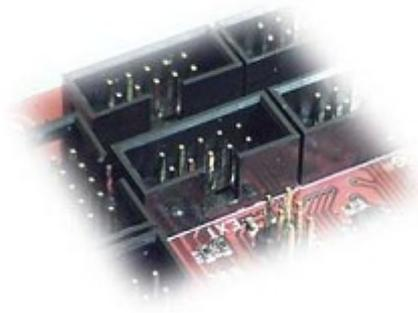
This connector allows use of SD Card and I2C protocol devices. An inexpensive I2C LCD digital readout has been successfully prototyped, tested and documented.
