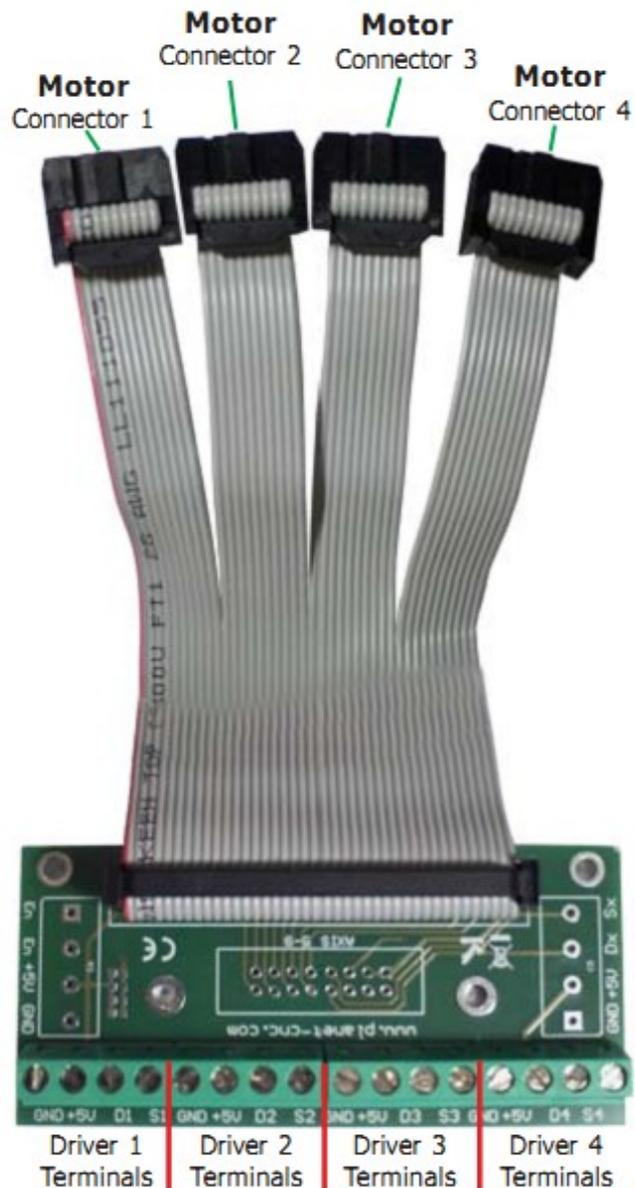
The Screw Terminal Adapter assists Mk1 and Mk2 controller connect to motor drivers that use screw terminal inputs. The adapter is compact. The ribbon cable connector helps in keeping enclosure wiring neat and accessible. Use is not difficult.
