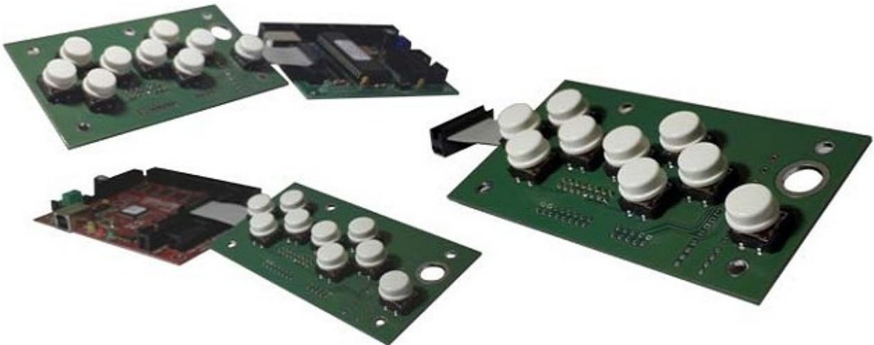
The jogging keyboard is a quick, easy and inexpensive means to add dedicated manual jogging buttons to Mk1, Mk2 and Mk2/4 CNC USB controllers.
