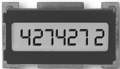
The single-channel count module type 190 for PCB mounting, with 2 voltage ranges (4.75 ... 15 and 9 ... 60 V DC) and large 7-digit LCD display, boasts a very wide temperature range.
