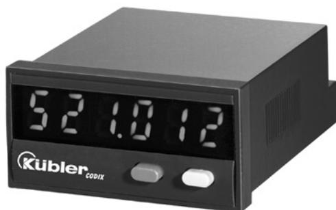
The Codix 52T is a voltage powered dual pulse counter with a common input and separate scaling, for fast and slow count pulses, with 6-digit LED display for NPN, PNP input signals and display switching between A and B.
