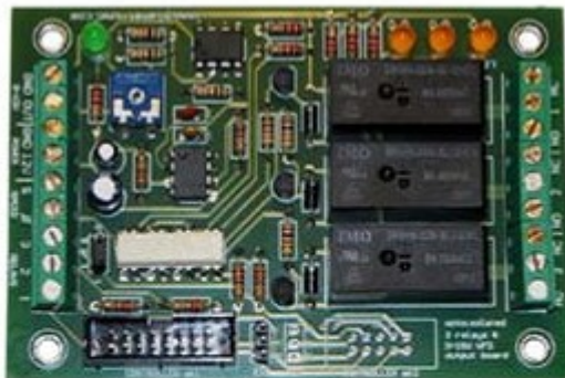
Output Board Adds Relays and VFD
